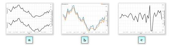
Figure 2.8: Design strategies for comparing visualizations can be subdivided into three categories: Juxtaposition (a), Superposition (b) and Explicit Encoding (c) [GAW<sup>+</sup>11]. The two compared Temperature 01 and Temperature 02 time series are from the used example data set (see Section 1.1) and are visualized with VISPLORE.
