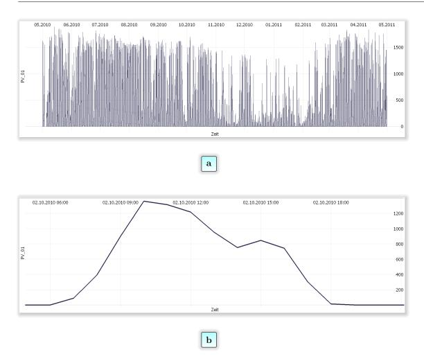
Figure 1.1: Photovoltaic power Production Values (PV). (a) shows the PV\_01 for the whole available time interval. (b) shows a single day.
