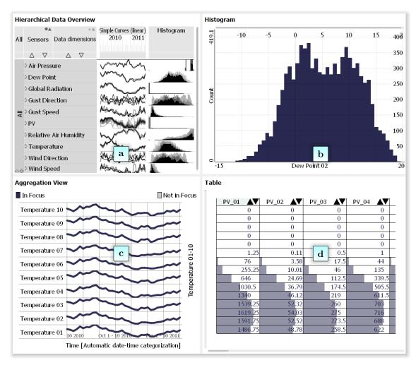
Figure 7.4: An example of multiple connected views in the software VISPLORE. This includes the presented HDO framework (a), Histograms (b), Time series (c) and detailed information (d).
