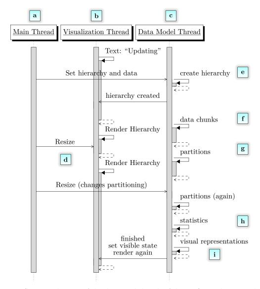
Figure 7.5: Sequence diagram of the three used threads of the HDO visualization. The main thread (a) waits for the user input (d). The visualization thread (b) renders the state. The data model thread (c) performs heavy computations (e–i).
