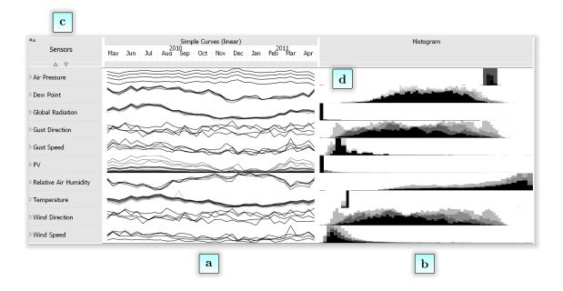
Figure 6.2: The HDO framework visualizes the time curves (a) and the distributions (b) of all 163 data dimensions combined by their sensors (c). (d) shows an outlier in the Air Pressure data
